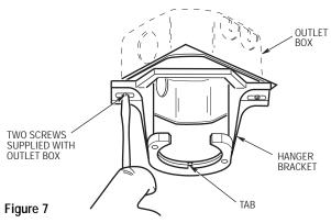
10. Carefully lift the fan and seat the hanger ball/downrod assembly on the hanger bracket that was just attached to the outlet box (Figure 8). Be sure the groove in the ball is lined up with tab on the hanger bracket (Figure 7).
